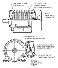
selection For and setting of suitable dependent current protection the t<sub>F</sub> time and the ratio of locked rotor current to nominal current are used. In the case of a rotor locking, this device must cut off the supply within the specified  $t_{_{\rm F}}$  time, which is listed in the performance data.
