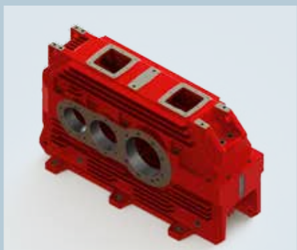
Gray cast (GG25) housing with extend- ed surface for better heat dissipation
